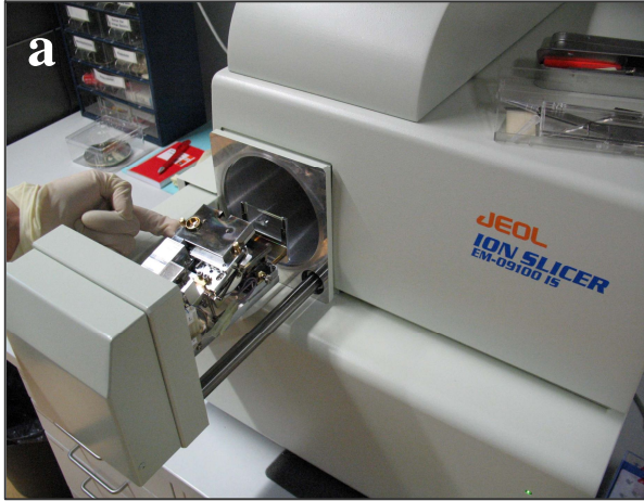
Figure 4. a. Argon Ion Slicer at GUF. b. Sample for TEM analysis, prepared by the Argon Ion Slicer.
