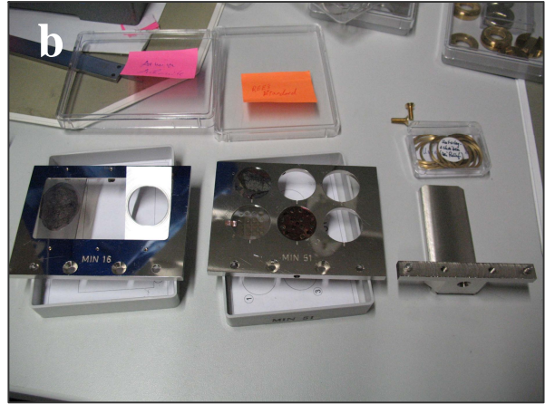
Figure 1. a. Laboratory for EMPA of GUF. b. Sample holders for EMPA.
