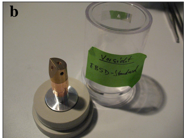
Figure 2. a. EBSD detector attached on the SEM of GUF. b. Sample holder for EBSD analysis.
